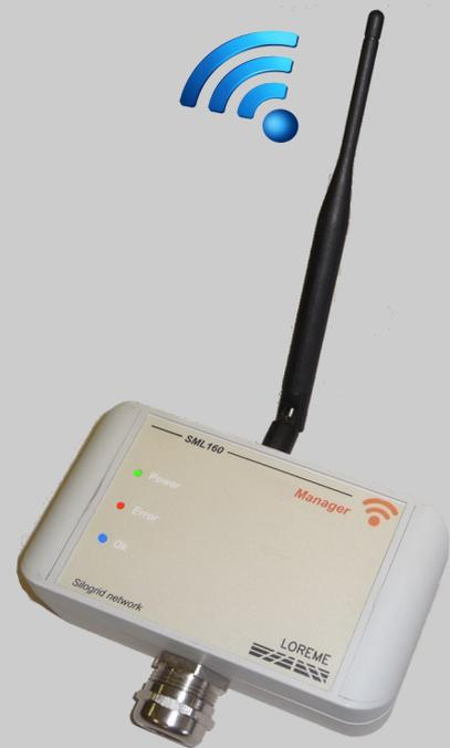
The SML160 is a wireless receiver with an Ethernet connection, the product centralizes all measures issued by the radio transmitters, and makes them available through a standard communication protocol (Modbus-TCP) on the Ethernet link.
