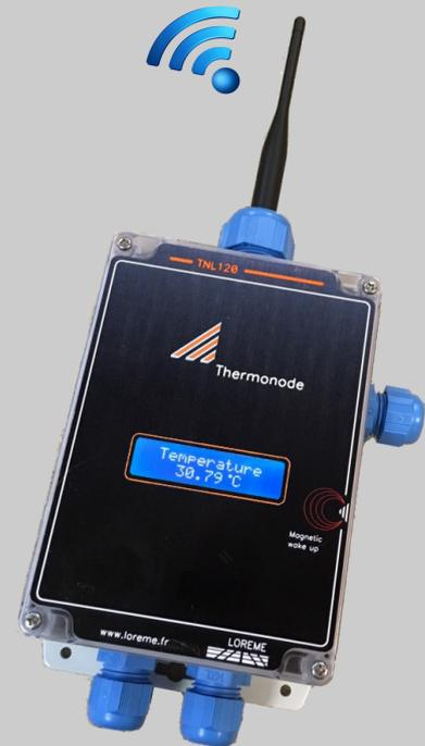
The TNL120mA is an autonomous and waterproof acquisition station, capable to broadcast the 4..20mA signal measurement by radio link. All transmitters form a mesh network with up to 32 stations. The measures are available via a Ethernet Modbus TCP link on manager (SML160mA).
